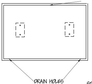
FRAMES ATTACH TO SURFACE WITH THRU BOLTS - PROVIDED
